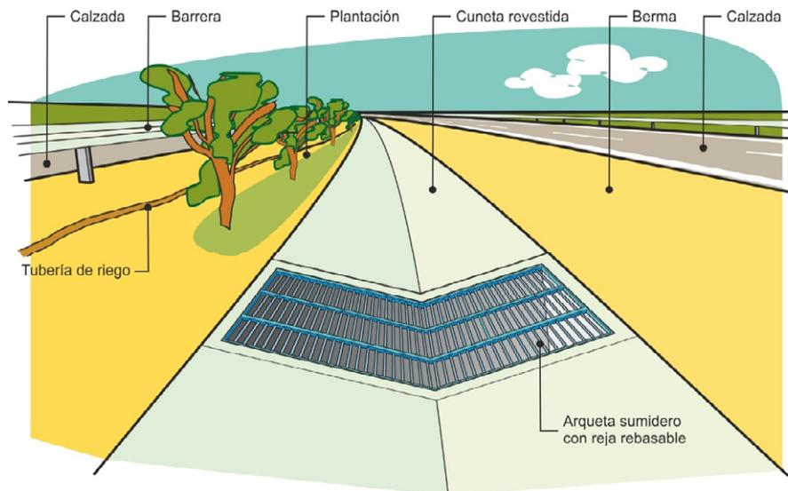
FIGURA 3.10 EJEMPLO DE CUNETA EN MEDIANA AMPLIA
