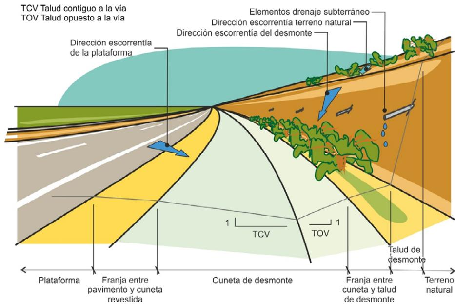
FIGURA 3.16 EJEMPLO DE CUNETAS EN MARGEN DE DESMORTE
