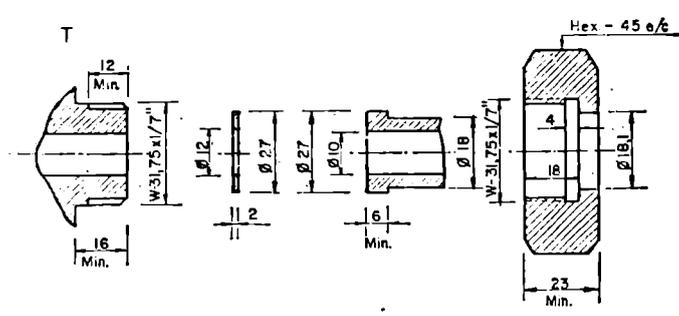
ACOPLAMIENTO W31,75 - 7 Hilos/Pulgada (DERECHAS) TIPO CLORO (BOTELLONES)
