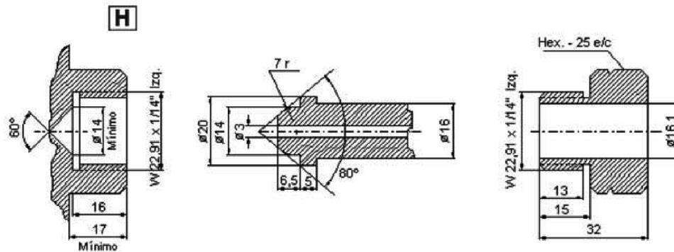
ACOPLAMIENTO W 22,91 - 14 Hilos/Pulgada (IZQUIERDAS).
