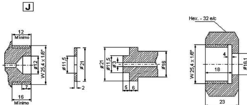
ACOPLAMIENTO W 25,4 - 8 Hilos/Pulgada (DERECHA).
