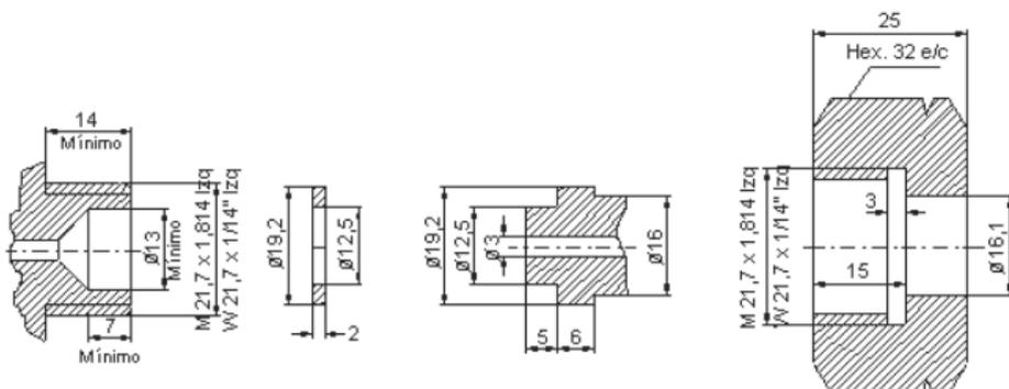
ACOPLAMIENTO M.21,7 x 1,814 METRICO (IZQUIERDAS)
