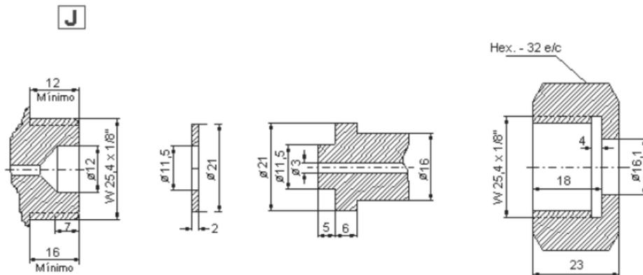
ACOPLAMIENTO W 25,4 - 8 Hilos/Pulgada (DERECHA)
