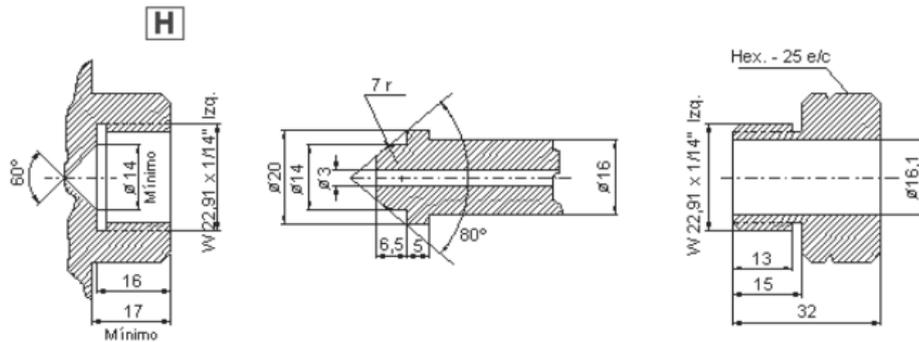
ACOPLAMIENTO W 22,91 - 14 Hilos/Pulgada (IZQUIERDAS)
